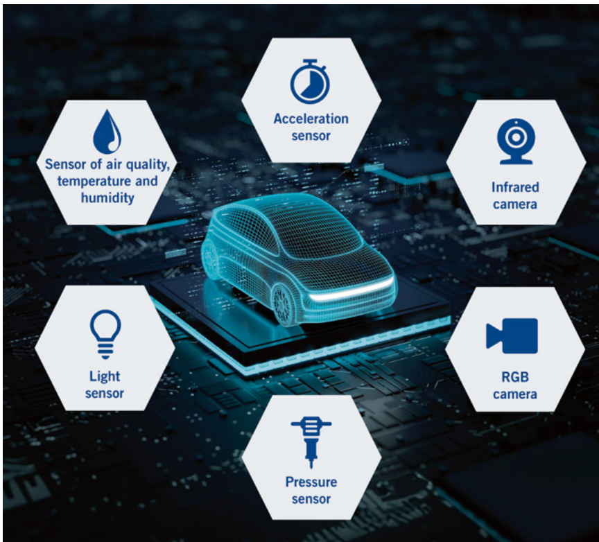
FIGURE 1 Types of interior sensors (© cono0430 | Shutterstock | ITK Engineering)
